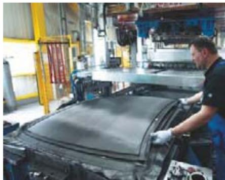
The Cannon preformer is in full production today supplying all the roof preforms required by the M3 and M6 models.
