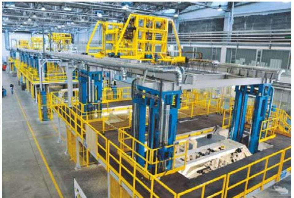
Above: Aermacchi - Alenia complex handling system designed and built by Cannon Tecnos to move the assembly jigs from one fitting station to the next ones where the fuselage of the new M-346 aircraft is assembled. Below: The new Aermacchi M-346 on the tarmac in Venegono Superiore, Italy.
