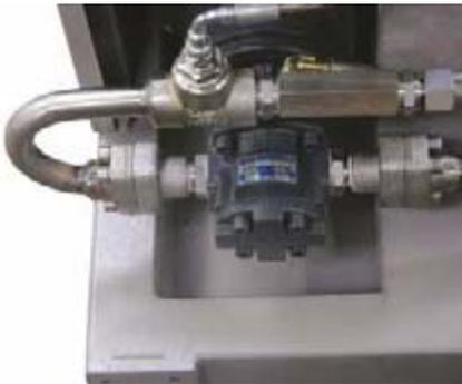
Special pumps are used for both Epoxy resin and hardener to guarantee high precision and reliability.
