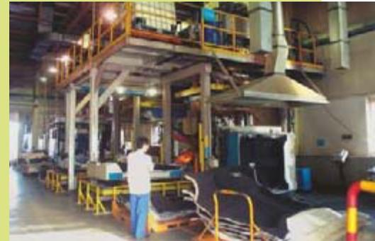
Cannon Tecnos modular carpet back foaming plant featuring metering system, pouring robot, mould clamps working in tandem and complete set of safety system.
