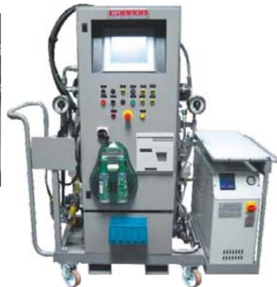
Epoxy DX35T including thermoregulation unit for resin
