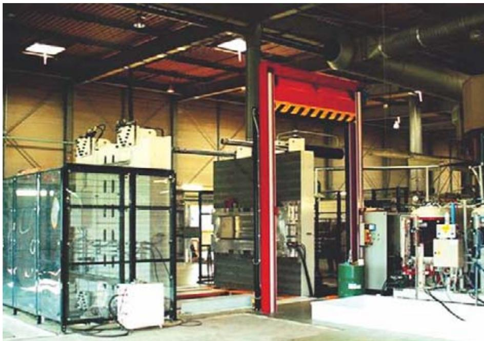
Hutchinson use a horizontal clamping press with a platen of 3,500 by 3,500mm, a stroke of 3,600mm and a clamping force of 230 Tons to process PDCPD (PolyDiCycloPentaDiene) resins.
